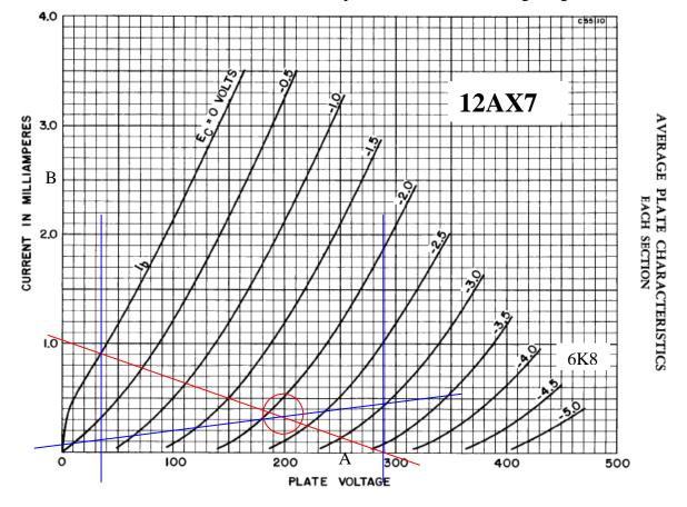
Cold biased for noticeable second-harmonic compression distortion on larger signals.
